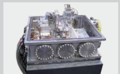
Interior of MAXYMUS. The beam enters from the left and is detected with a detector system at the right.
